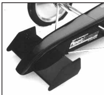
Without inner tip plates for profile fit to body.
